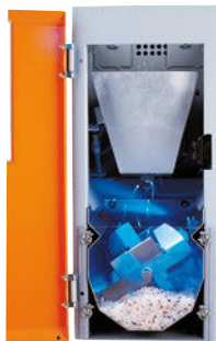
Weigh bin and mixing chamber
