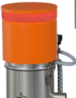
METRO SG HES / alarma encendida
