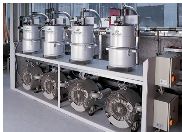
Central vacuum station
